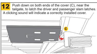
Preferred method of closure: Close tailgate, then close cover on top of tailgate. This method will not work with some truck applications. Use alternative method instead.
