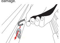
To release strap push tab up. **NOTE:** Ice buildup within hinge sections can occur if cover is stowed in open position. To prevent potential damage, close cover during winter precipitation.
